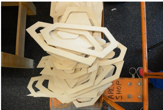
[Figure 66] The final Plywood frames. These frames go on top of the latex rubber sheets to form the inflatable bladders. On the right both the wooden frames and the MDF base are shown. (Author, 2017)
