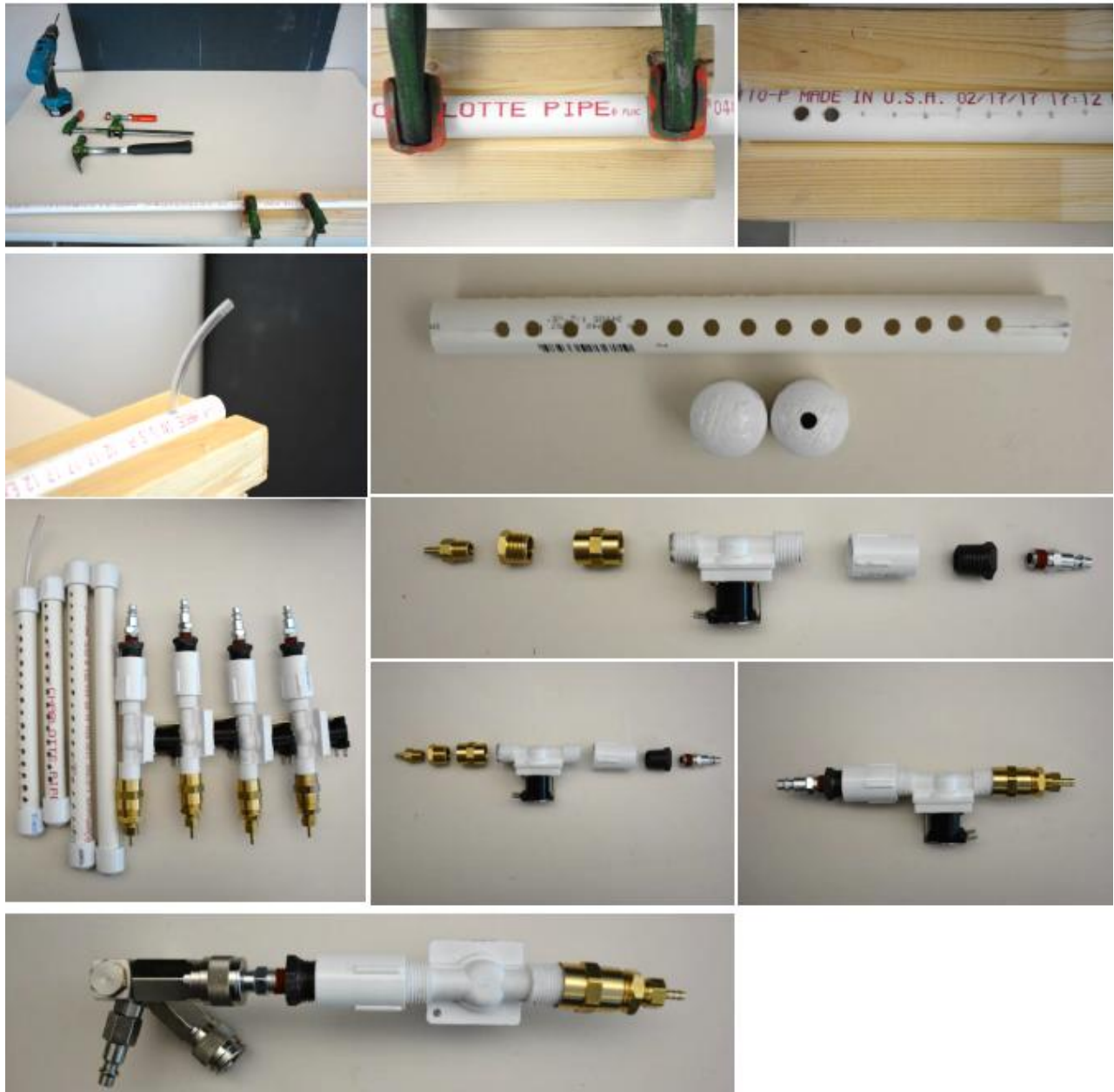
[Figure 79] The Process for making the manifolds and details for connecting manifolds to the solenoid valves. (Author, 2017)
