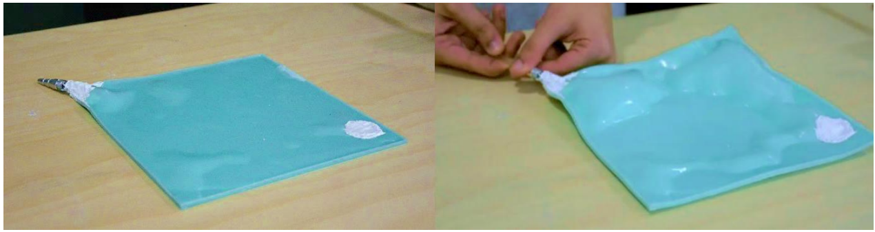
[Figure 31] Inflatable prototype. Left: the double layer silicon that has not yet been inflated. Right: Channeling air through the casted silicon for inflation and shape-change. (Author, 2017)
