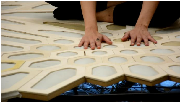
[Figure 82] The prototype's behavior towards user's presence. The bladders inflate and deflate one zone after another in the area where the body is detected. (Author, 2017)
