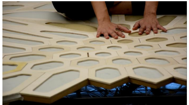
[Figure 82] The prototype's behavior towards user's presence. The bladders inflate and deflate one zone after another in the area where the body is detected. (Author, 2017)
