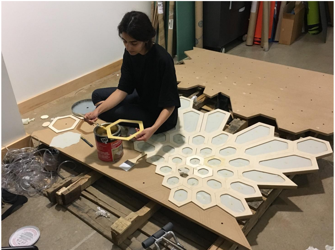
[Figure 73] Sitting on the floor prototype, the latex rubber is glued to the MDF and the frame is glued on top of the latex rubber using contact cement. In this Image almost half of the floor is ready to be inflated. (Author, 2017)
