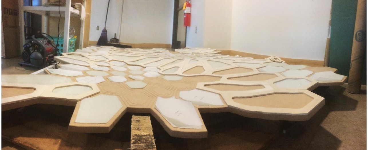
[Figure 69] All of the pieces were tested on the platform to make sure all pieces are in place. However, unfortunately, I came short on latex rubber and had to fill in some of the bladders. (Author, 2017)
