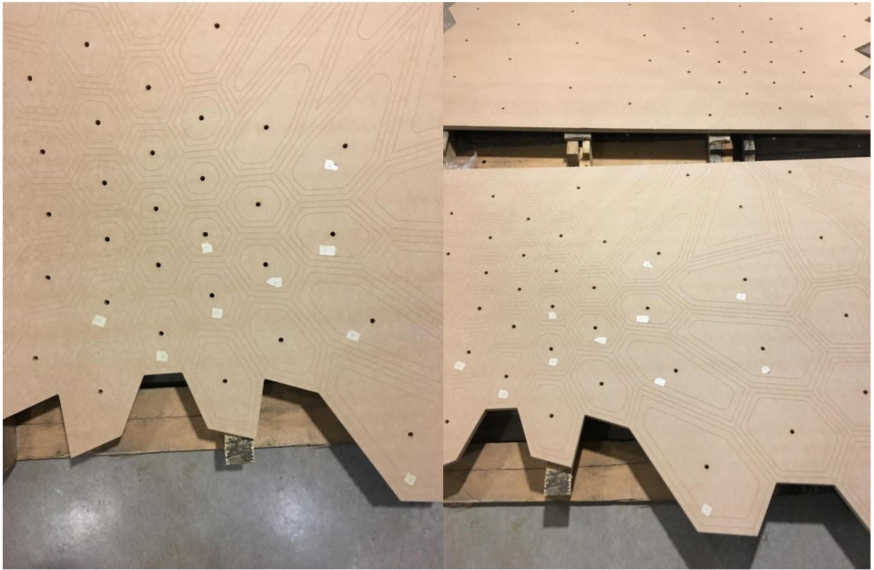
[Figure 71] The holes are cleared to fit the 1/4" air tubing. (Author, 2017)
