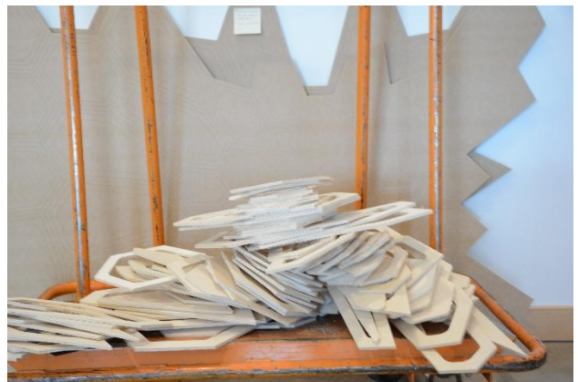
[Figure 66] The final Plywood frames. These frames go on top of the latex rubber sheets to form the inflatable bladders. On the right both the wooden frames and the MDF base are shown. (Author, 2017)
