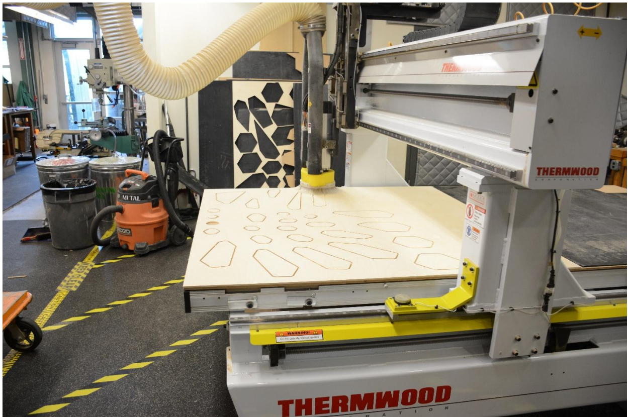
[Figure 63] The CNC is cutting through the Ply wood as the frame for the inflatable structure. The CNC Machine is located in the ground floor at the Stuckeman School of Architecture and Landscape Architecture at the Pennsylvania State University. Easy access to the machine made this process much more convenient. (Author, 2017)
