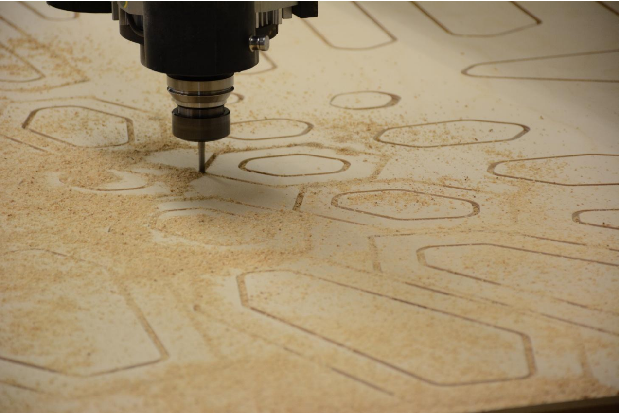
[Figure 65] The CNC Machine is cutting the inner lines of the frames. The brush has been removed for a clearer cut on the smaller pieces. (Author, 2017)
