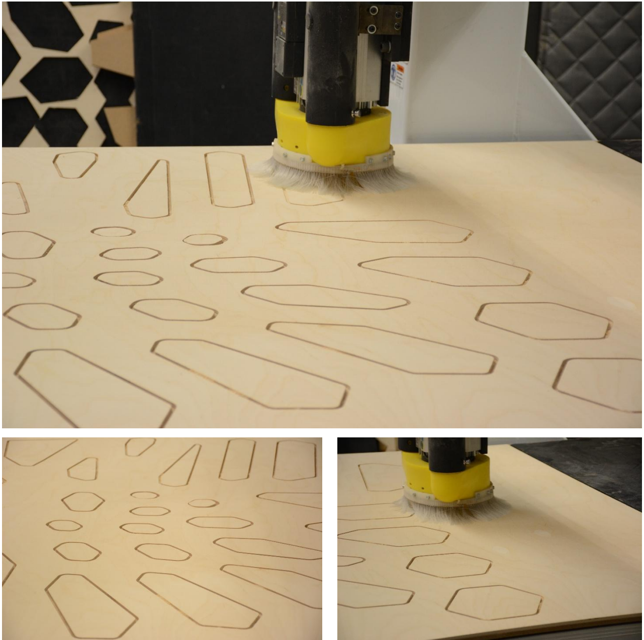
[Figure 64] The CNC machine cutting the outlines. (Author, 2017)
