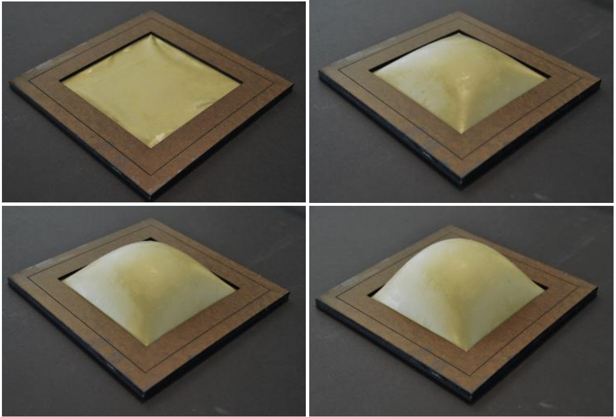
[Figure 33] Flat and Inflated version of the latex rubber prototype compressed between two layers of Masonite. 10 PSI air pressure was enough for inflating this prototype unit. (Author, 2017)
